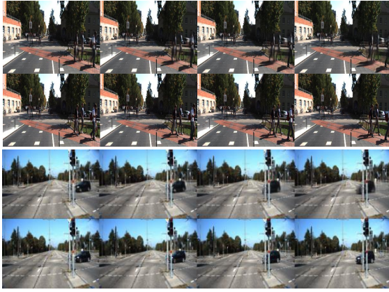
Fig. 5. 4-step short-term prediction on KITTI. In each group, the first row indicates the predicted result and the second row indicates the ground truth.
